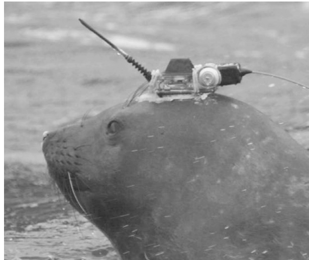
FIG. 1. CTD–SRDL deployed on a southern elephant seal. An additional VHF tracking device is attached on the back.
