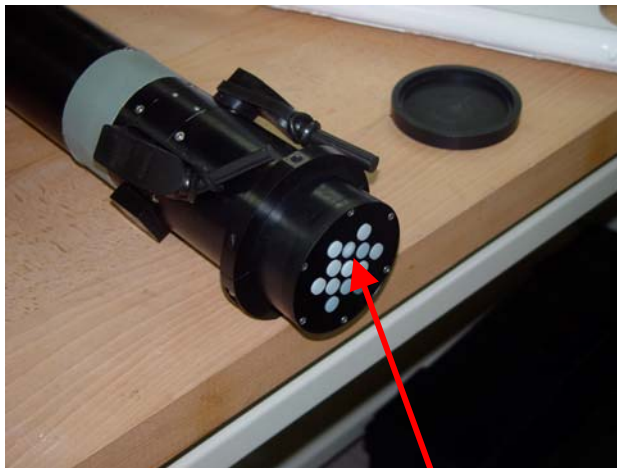
The SMSR head, with the 13 cosine collectors
